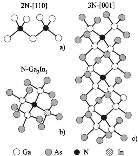
**Fig. 3** Ball and stick models of different N configurations in  $\text{Ga}(\text{NAs})$  and  $(\text{GaIn})(\text{NAs})$ : (a) N nearest neighbor in [110] direction; (b) N in a 3Ga 1 In configuration; and (c) N chain, oriented in [001] direction
