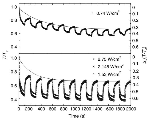
**Fig. 5** Fitting of the photodarkening measurements at room temperature to the Eq. 6 (solid lines). Upper part ( $I = 0.74 \text{ W/cm}^2$ ):  $\tau_{ir} \cong 400 \text{ s}$ . Lower part ( $I \geq 1.53 \text{ W/cm}^2$ ):  $\tau_{ir} \cong 200 \text{ s}$
