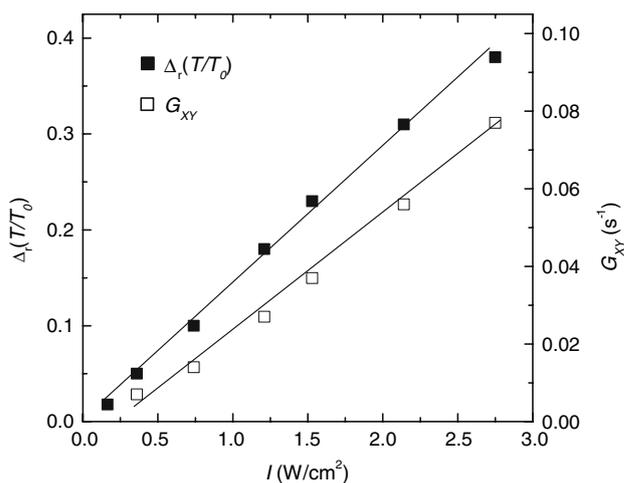
**Fig. 4** The magnitude of the reversible PD effect (filled squares) and the conversion rate from the ground state configuration X into the configuration Y responsible for reversible PD component (open squares) as function of the light intensity
