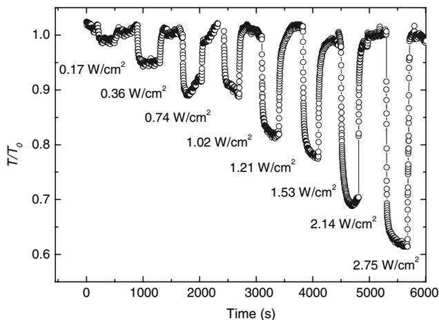
**Fig. 3** Photodarkening measurements at 35 °C for eight different light intensities. The light intensity was kept constant at the level indicated for each cycle consisted of 500 s of pumping followed by 500 s of rest
