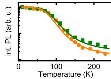
FIG. 4. (Color online) Temperature dependence of the PL intensity. The solid lines represent the simulation and squares/dots show the measured normalized PL intensity for  $N_{nr}/(N_r + N_{nr}) = 0.012$  and excitation power  $P = 5$  mW (lower curve), and  $N_{nr}/(N_r + N_{nr}) = 0.008$  and  $P = 10$  mW (upper curve).
