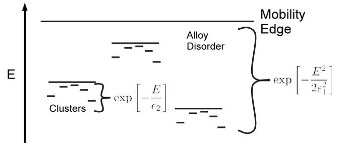
FIG. 2. Hopping on two energy scales. The first one is given by a Gaussian distribution with the characteristic energy scale  $\epsilon_1$  and the second scale is given by an exponential distribution with energy scale  $\epsilon_2$ , representing alloy disorder and cluster localization, respectively.
