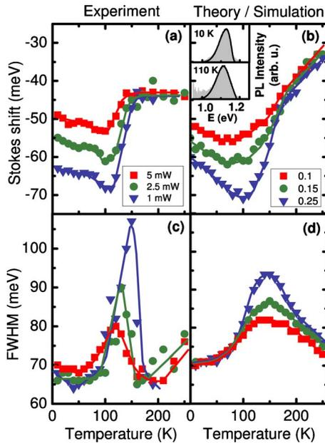
FIG. 3. (Color online) Left: Experimental Stokes shift (a) and FWHM (c) for varying excitation powers. Right: Calculated Stokes shift (b) and FWHM (d) for varying  $N_2\alpha_2^2$  using the two-scale model. Energy scales of  $\epsilon_1 = 45$  meV and  $\epsilon_2 = 11$  eV are obtained. The inset in (b) shows experimental (gray area) and theoretical (black line) PL spectra for the temperatures of 10 and 110 K at the excitation density of 1 mW.
