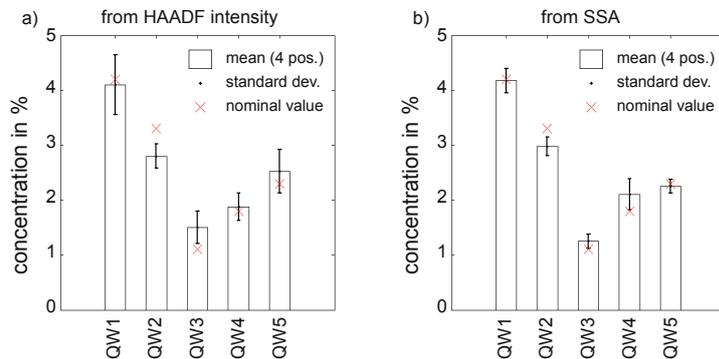
**Figure 3.** Concentrations measured for all five QWs a) by evaluation of HAADF intensity and b) from strain state analysis. Shown are the mean values of four evaluated areas in each case. The errorbars represent the standard deviations and do not contain the error of the single measurement.
