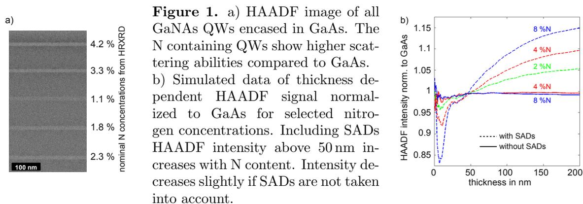
imaged GaAs should be brighter compared to the nitrogen containing QW (e.g. observed by Herrera *et al.* [9]). However, taking SADs into account, we observe a different behavior: for typical STEM specimen thicknesses above 50 nm, the HAADF signal increases with nitrogen concentration. Figure 1 b) shows the simulated HAADF intensity normalized to GaAs for selected concentrations.
